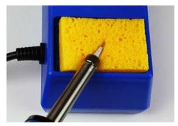
**Step 1:** Begin by making sure the tip is attached to the iron and **screwed tightly** in place.
