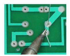
Step 2: Heat the Joint – Turn your soldering iron on and if it has an adjustable heat control set it to 400°C. At this point, touch the tip of the iron to the copper pad and the resistor lead at the same time. You need to hold the soldering iron in place for 3-4 seconds in order to heat the pad and the lead.
