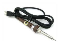
You won't get far into a soldering project without a soldering iron. This is a hand tool that plugs into a standard 120v AC outlet and heats an interchangeable metal tip up to a very hot 896° F in order to melt solder. Soldering irons come in several varieties, including pen or gun type. We recommend that you use a pen type soldering iron in the 15W to 30W range when you're learning to solder.
