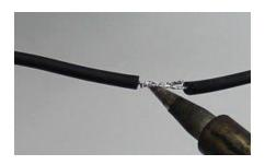
**Step 4:** Hold the two tinned wires on top of each other and touch the soldering iron to both wires. This process should melt the solder and coat both wires evenly.
