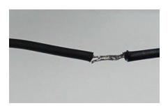
**Step 5:** Remove the soldering iron and **wait a few seconds** to let the soldered connection cool and harden. Use heat shrink to cover the connection.
