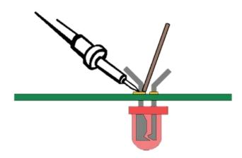
If you were to take apart any electronic device that contains a circuit board, you'll see the components are attached using soldering techniques. **Soldering** is the process of joining two or more electronic parts together by melting solder around the connection. Solder is a metal alloy, and when it cools it creates a strong electrical bond between the parts. Even though soldering can create a permanent connection, it can also be reversed using a desoldering tool.
