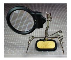
A helping hand is a device that has 2 or more alligator clips and sometimes a magnifying glass/light attached. These clips will assist you by holding the items you are trying to solder while you use the soldering iron and solder.
