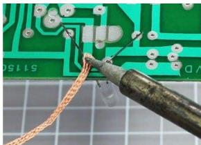
**Step 1:** Place a piece of the desoldering braid on top of the joint/solder you want removed.
