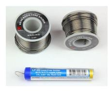
Some examples of rosin-core solder. It comes in a variety of diameters and metallic formulations. Be sure you buy the *rosin-core* variety; solid-core will be much harder to work with and require you to buy flux, while acid-core may damage your circuits and components!
