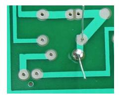
Step 4: Snip the Leads – Remove the soldering iron and let the solder cool down naturally. Don't blow on the solder as this will cause a bad joint. Once cool, you can snip the extra wire from leads. A proper solder joint is smooth, shiny, and looks like a volcano or cone shape. You want just enough solder to cover the entire joint but not too much so it becomes a ball or spills to a nearby lead or joint.
