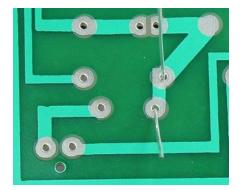
Step 1: Mount the Component – Begin by inserting the leads of the LED into the holes of the circuit board. Flip the board over and bend the leads outward at a 45° angle. This will help the component make a better connection with the copper pad and prevent it from falling out while soldering.
