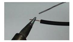
**Step 3:** Keep the iron in place and touch the solder to the wire until it is **fully coated**. Repeat this process on the other wire.
