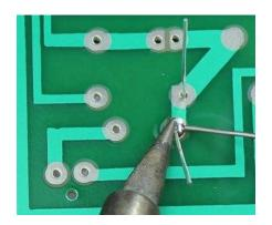
**Step 3: Apply Solder to Joint** – Continue holding the soldering iron on the copper pad and the lead and touch your solder to the joint. **IMPORTANT** – Don't touch the solder directly to the tip of the iron. You want the joint to be hot enough to melt the solder when it's touched. If the joint is too cold, it will form a bad connection.
