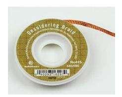
To desolder a joint, you will need solder wick, which is also known as desoldering braid. It is essentially copper wire that is braided together and dipped in flux to allow it to absorb solder with the application of heat. Solder wick is particularly helpful when hand-reworking boards with surface-mount devices (SMDs), as the wide contact area and absorbing action is very useful for cleaning the small copper pads that surface-mount integrated circuits connect to.
